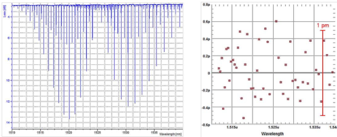
Figure 4. Deviation of C<sub>2</sub>H<sub>2</sub> absorption wavelengths from literature, measured at 200 nm/s sweep speed
