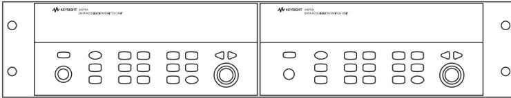
To rack mount two instruments side-by-side, order 34191A 2U dual flange kit and 34194A dual lock link kit.
