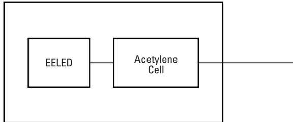
Figure 1. Wavelength calibrator block diagram
