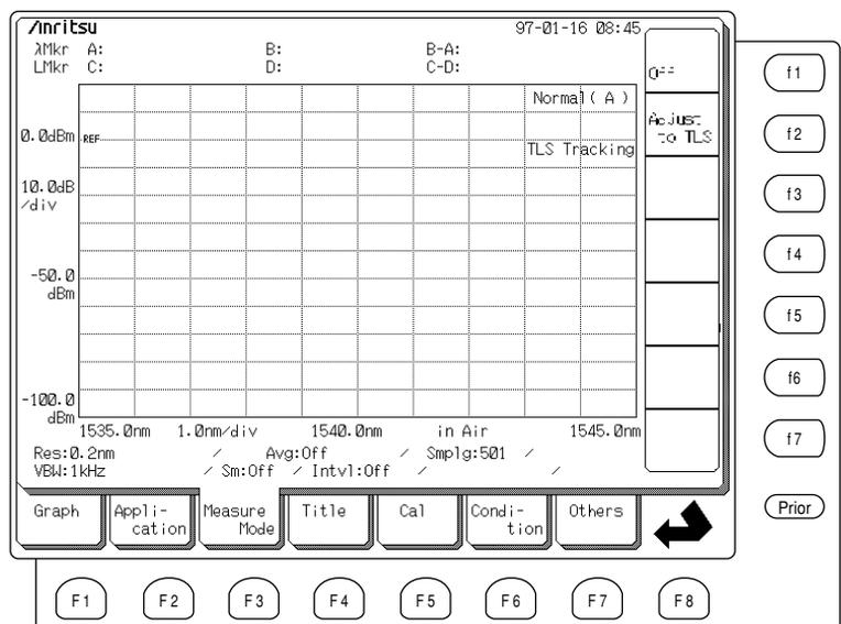
If the message “TLS Interface Error” is displayed at this time, check the cable connections again and the MG9637/MG9638 settings.
