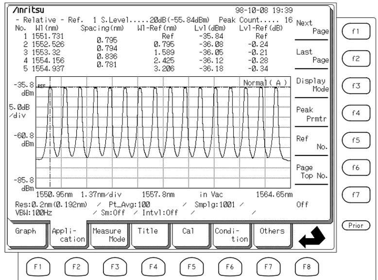
In the Relative mode, the wavelength, level, and wavelength spacing, or the wavelength and level relative to a reference peak, can be displayed for up to 5 peaks simultaneously.
