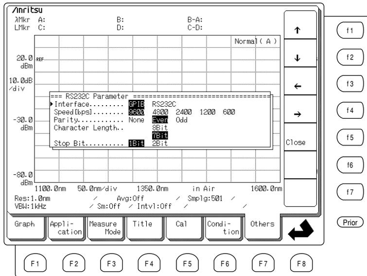
The following function keys are displayed in the Functions display field at right-hand side of the screen. Use the function keys to select the item indicated by the reverse displayed cursor.
