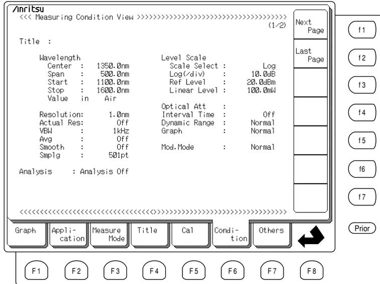
On this screen, press the Next Page function key **f1** to display the system setting conditions as shown below. To return to the measurement conditions screen, press the Last Page function key **f2**.
