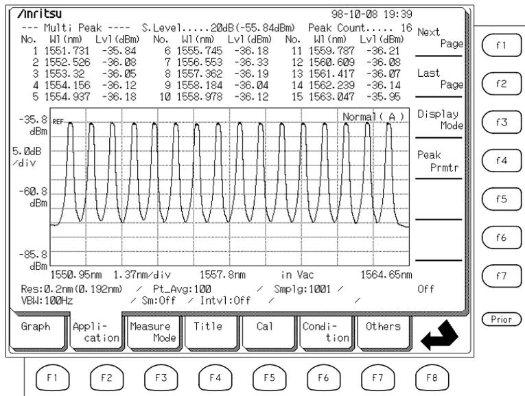
In the Multi Peak Mode, the wavelength and level of up to 15 peaks can be displayed simultaneously. Next page displays the following page.
