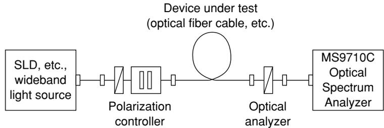
Convert the light from a wideband light source to a polarized wave using a polarization controller; pass this polarized light through the device under test, and input it to the MS9710C through an analyzer. The MS9710C measures the optical power polarization wavelength changes and calculates the PMD.
