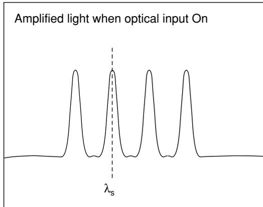
Measurement is performed with automatic evaluation whether or not wavelength of the optical signal is modulated by switching the optical input On and Off.
