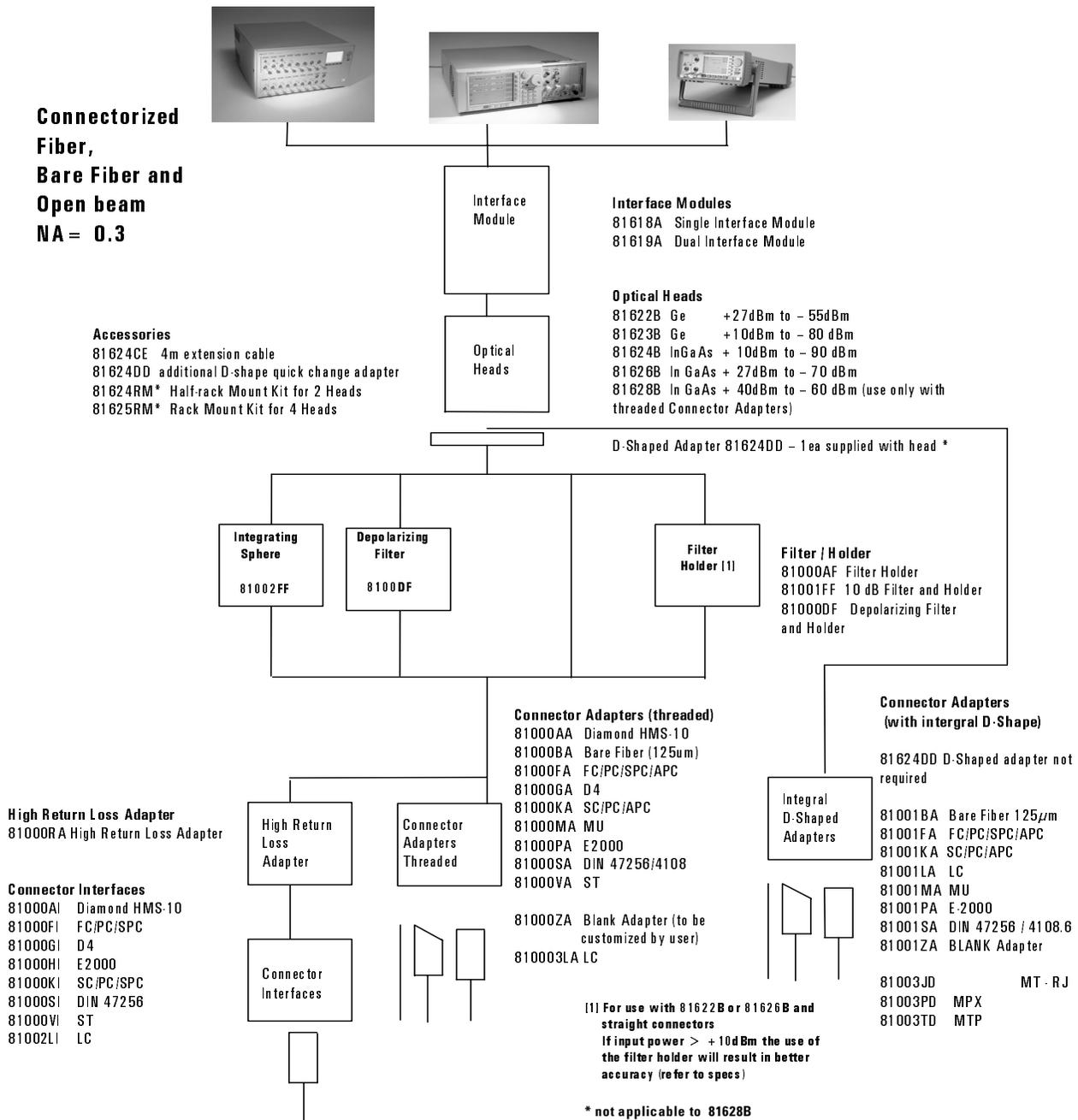
Figure 7 Optical Head Accessories (5 & 3 mm Sensors)
