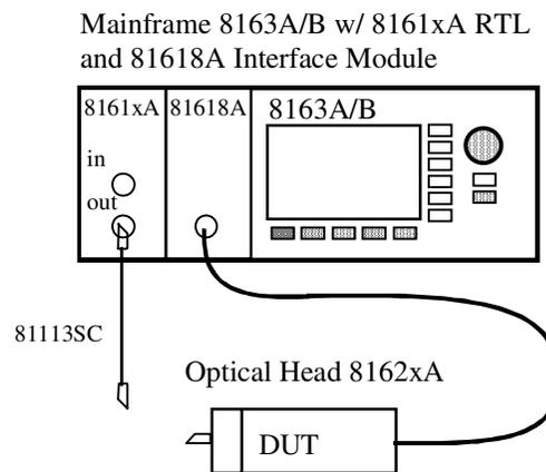
**Figure 14 Return Loss Measurement Setup**
