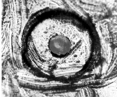
**Figure 3-7. Damage from improper cleaning.**
