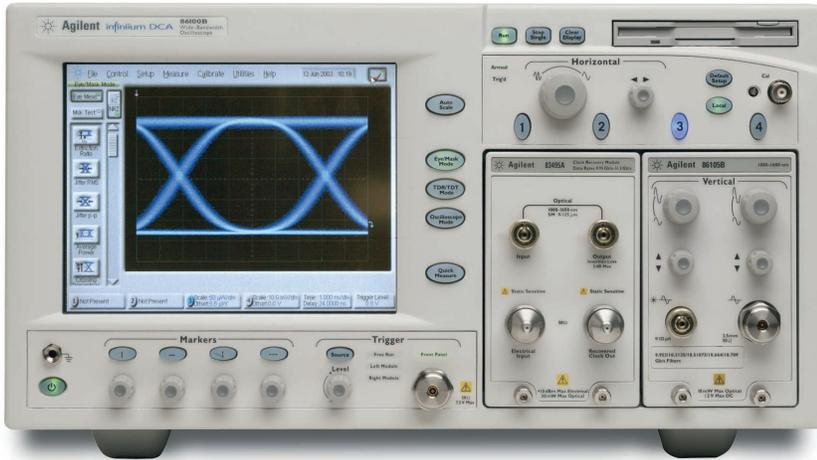
The 86105B and the 83495A make a low cost, flexible solution for 10 Gb/s testing.
