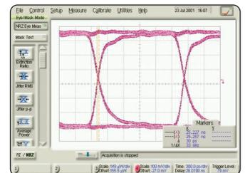
Identical incoming signals triggered with different loop bandwidths. The left one, triggered with the narrow loop bandwidth, reveals the presence of low frequency jitter on the data. The right one, triggered with a wide loop bandwidth, tracks out low frequency jitter making the signal appear much cleaner.
