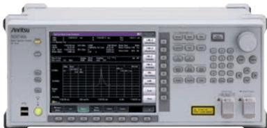
High-speed waveform sweeping and range processing support spectrum measurement at 0.2 s/5 nm.
