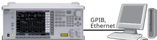
Data is transferred at high speed from waveform sweeping to external controller equipment.
